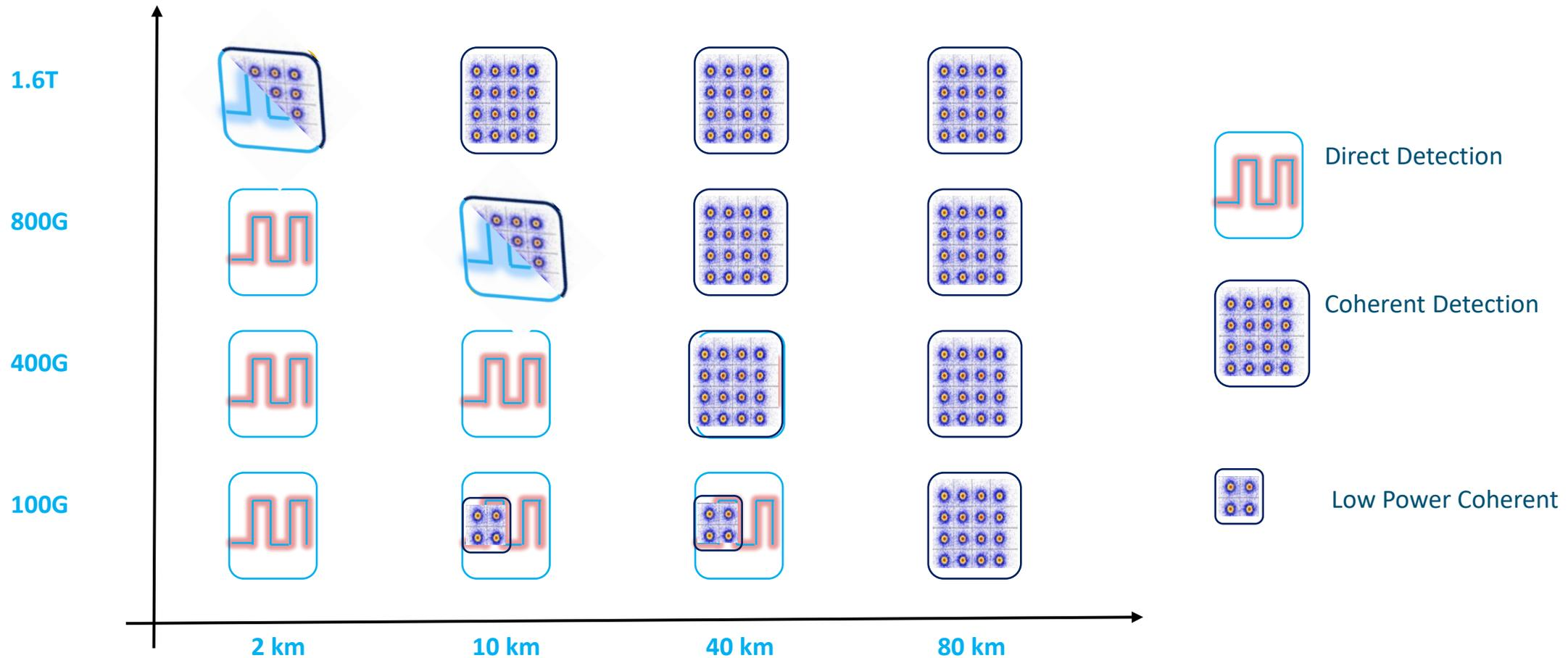
**Low Power Coherent 100G Replacing Nx10G in Short Reaches**
