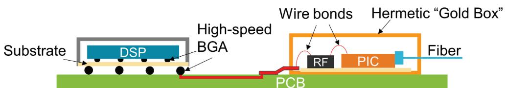
*Figure 3. Illustration of a conventional high-speed RF electrical interconnect between coherent DSP and PIC.*
